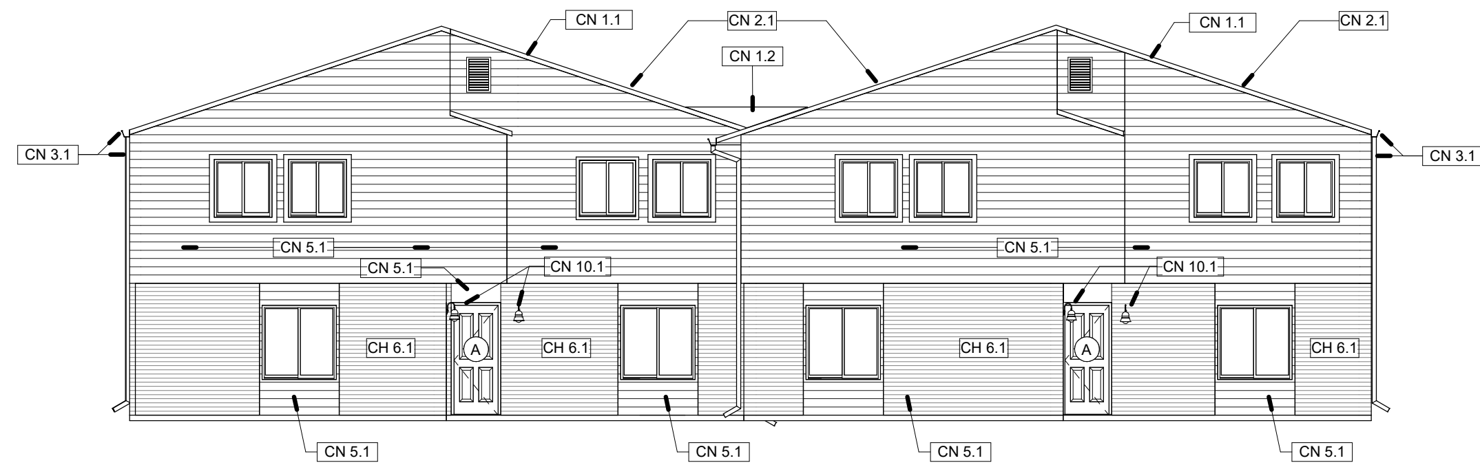
2 BUILDING TYPE III REAR ELEVATION 1/8" = 1'-0"
